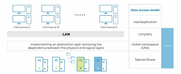
You can architect this File Area Network (FAN) using StorageX, an integrated suite of tools that logically aggregates distributed file data across heterogeneous storage environments and across CIFS- and NFS-based file systems, while providing policies to automate data management functions.
